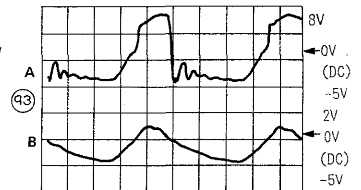
• D102 ANODE SIDE ( (93) -A) 5V/div. 2μs/div. • HIC101 pin (5) ( (93) -B) 5V/div. 2μs/div.
